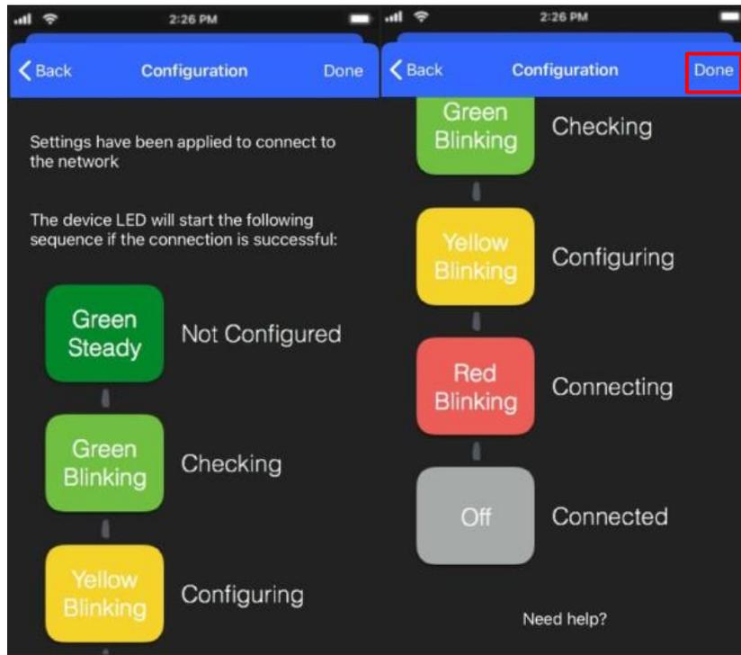
Figure 3.5 LED configuration network sequence.
