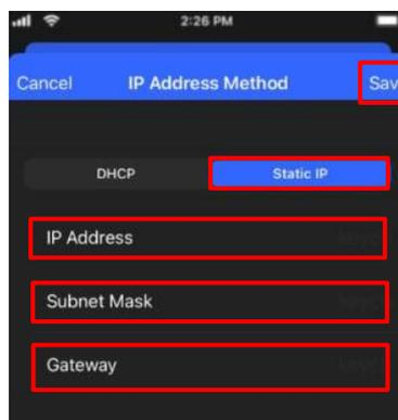
Figure 3.13 Advanced options (Static IP).
